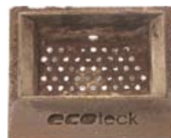
Burnpot needing cleaning with the holes blocked by ashes
